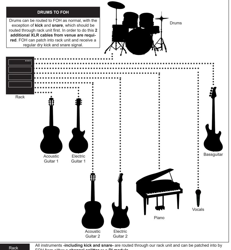
All instruments -including kick and snare- are routed through our rack unit and can be patched into by FOH from either a **channel splitter** or a **DI module**.
